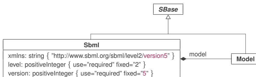
Figure 9: The definition of Sbml for SBML Level 2 Version 5 . The class Model is defined in Section 4.2. Note that both Sbml and Model are subclasses of SBase , and therefore inherit the attributes of that abstract class.
