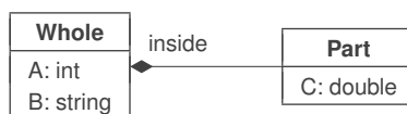
Figure 2: Example illustrating composite aggregation: the definition of one class of objects employing another class of objects in a part-whole relationship. In this particular example, an instance of a Whole class object must contain exactly one instance of a Part class object, and the symbol referring to the Part class object is inside . In XML, this symbol becomes the name of a subelement and the content of the subelement follows the definition of Part .
